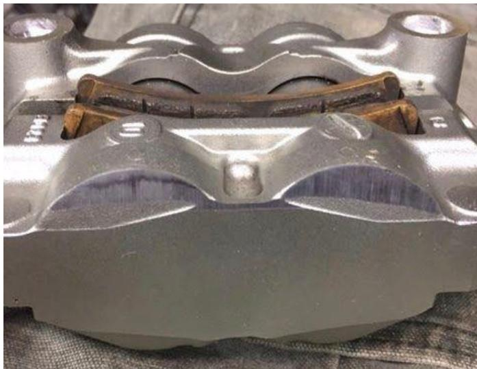
**Caliper Modification:** (*this should not be necessary for European 100mm Brembo calipers but may be required with other untested choices*). Using a file, block sander, or a grinder, Shave off 2mm of material at a 12 degree angle from the inside leading corner of the caliper, the corner closest to the spokes, to create at least 2mm of clearance. Do not remove so much material that the integrity of the caliper piston barrel is compromised.
