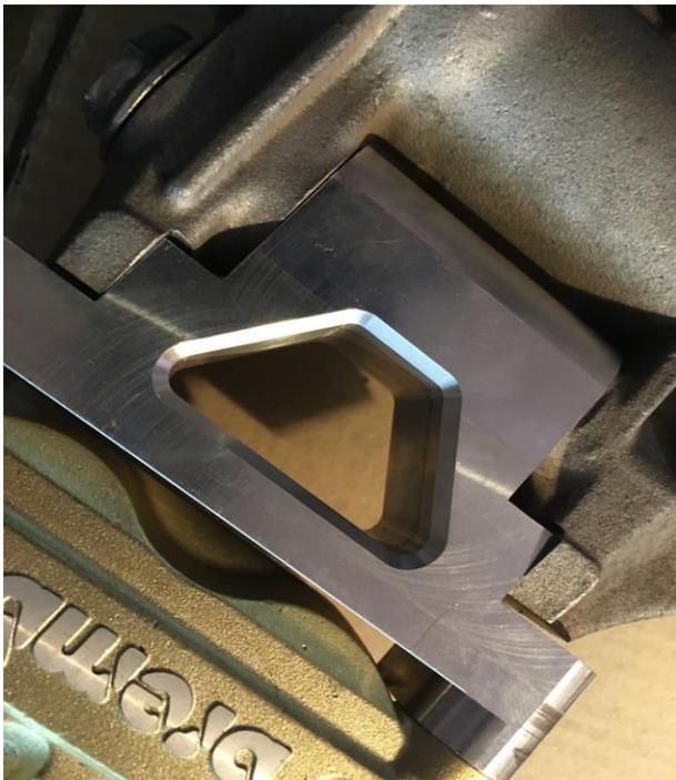
It is completely fine to have a gap between the adapter and the fork leg.
