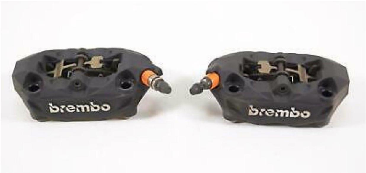
S1000RR Brembo radial 34mm 4 piston Calipers Provide the best clearance for spoke wheels. But will require an 18 to 19mm Master Cylinder for dual use. 13 to 15mm for single brake
