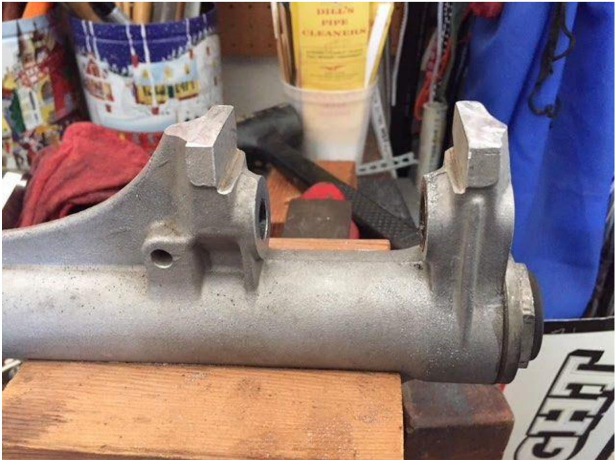
**For dual brake applications** it is relatively simple, with my modification process, to make a left fork lower into a much less common right leg slider. Because the legs are very symmetrical, after neatly modifying the leg as above, have a qualified machine shop enlarge the axle hole to snugly fit the large end with the clamp bolt loosened. I used this method for my R90/6.
