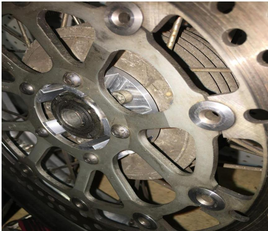
I supply Stainless bolts necessary for mounting the adapters. Position the hub adapter without the disc. Torque your long OEM BMW bolts to manufacturer spec. Mount the rotor and torque the 8mm rotor bolts to 9-10 ft/lbs and use blue Loctite.
