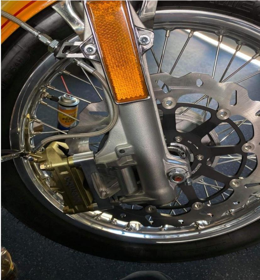
to prevent kinking. Routing of the line should allow the bars to turn freely without stressing the hose. Try several routes with some cheap plastic hose from the hardware store first before settling on a length. Another method that works is to have a short line made that couples to the main line and replaces the hard tube.
