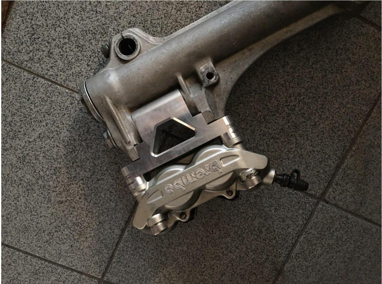
Brembo calipers are narrower than others, which is necessary to provide sufficient clearance for the spokes. There are even narrower calipers out there in the racing world, but because of expense I have yet to test any. Other Radial Calipers may work for European 100mm bolt pattern motorcycles, but have not been tested yet.
